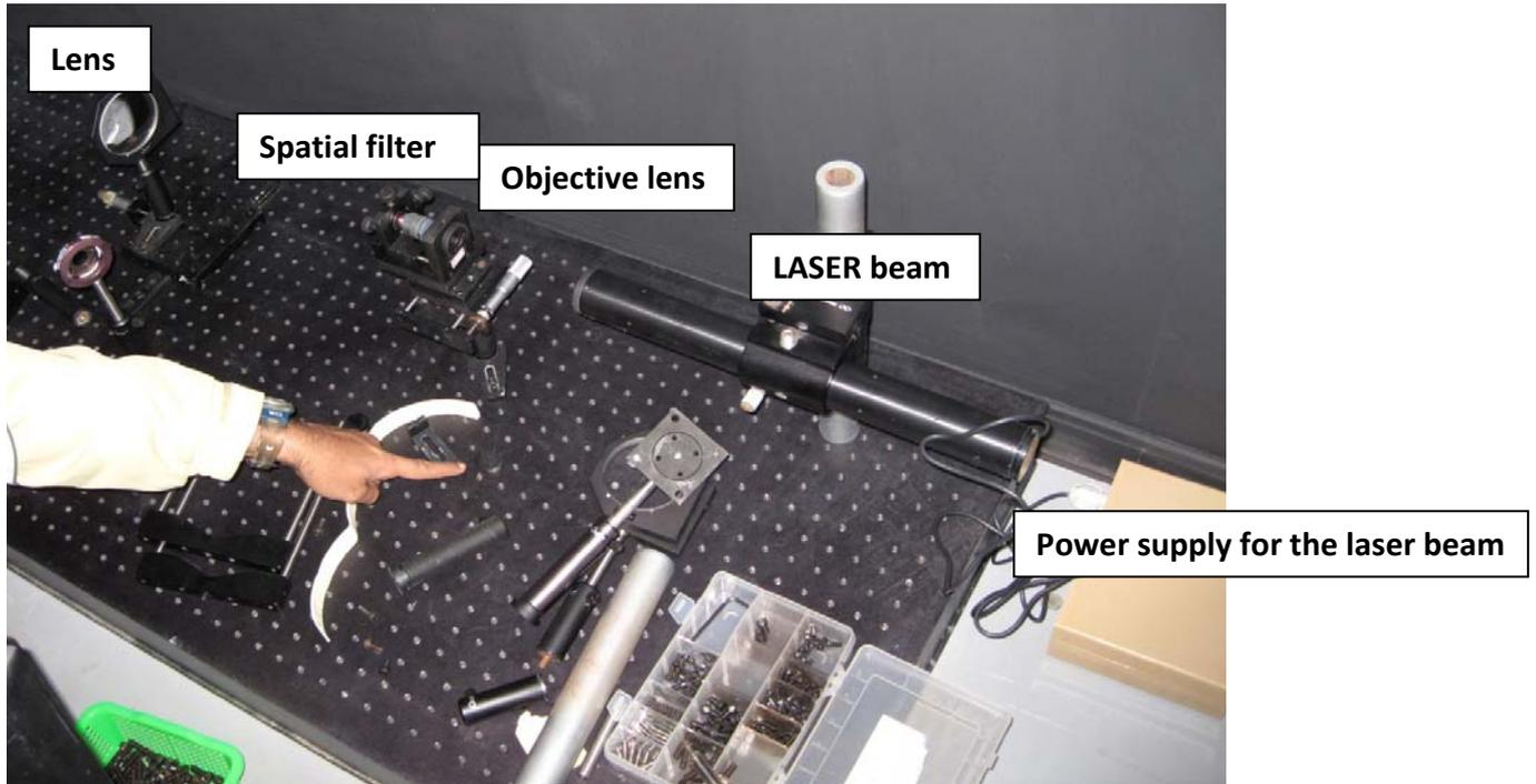
**Assembly for the Laser light equipment**
