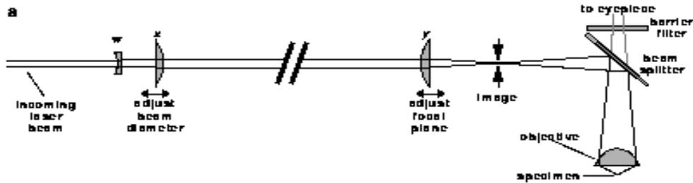
Lens y focuses the beam to a point within the image, so that it will focus to a corresponding point within the specimen. Lens y can be moved along the beam axis to adjust the focus of the laser so that it corresponds to the image you see. If it is moved toward the laser, the focus will move upward in the specimen. The laser light cannot be focused to a point in the image, because no image is formed. In this case one uses an additional lens (z in the figure) to form an image.
